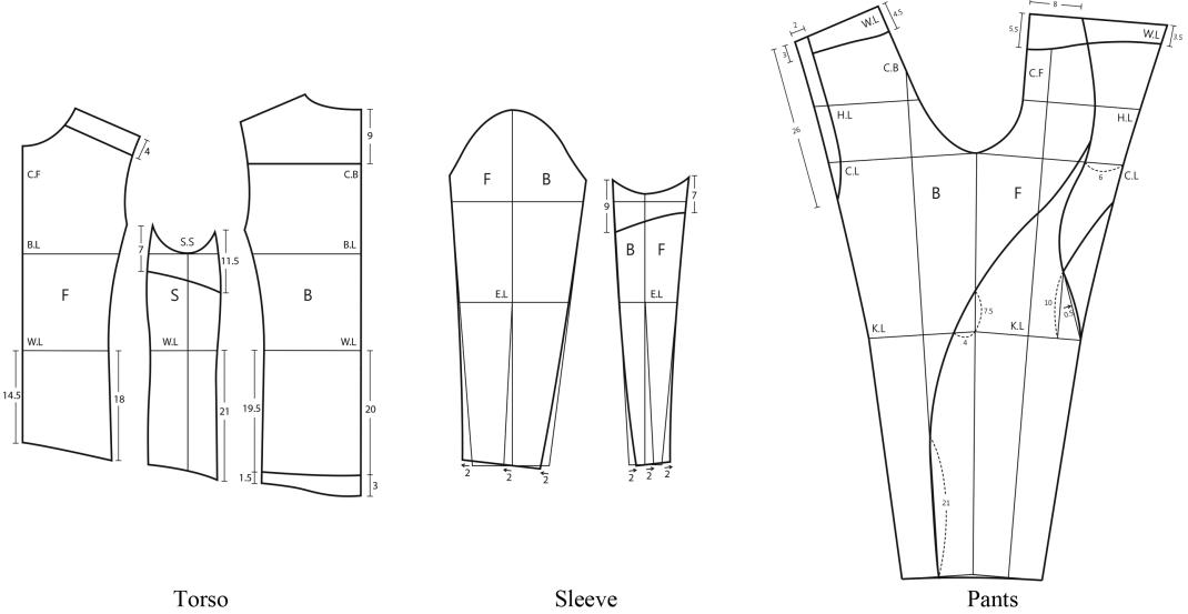
Fig. 6. Pattern making for bicycle wear.
